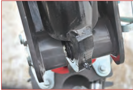
Spherical ball bushings isolate the cylinder alignment and increase the rotating bearing surface at the joint.
