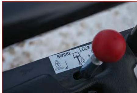
The swing lock prevents the boom from swinging during transportation.
