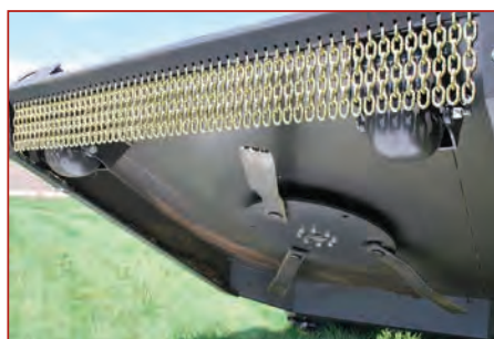
New .25" thick steel deck design.
