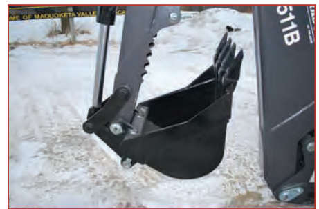
Heaped bucket capacities from 0.61 ft. 3 - 4.73 ft. 3 depending upon bucket selection.
