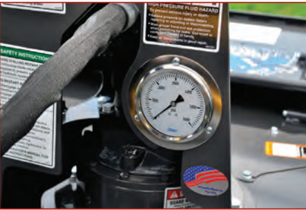
Standard pressure gauge indicator, easily visible to the operator helps prevent excessive stalling and overheating.
