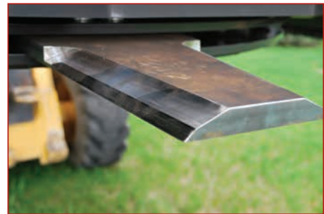
Four double bevel reversible edge blades.
