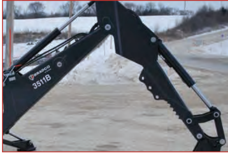
Cushioned cylinders for boom, dipper and swing provide smoother operation with less slamming and pressure spiking.
