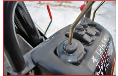
Easy controls - left lever runs boom and swing, right lever runs bucket and dipper while the middle levers run right and left stabilizers.
