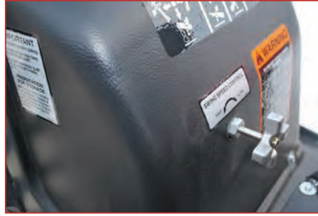
Swing speed control allows the operator to fully adjust the swing speed to the job.
