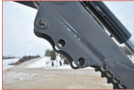
A standard thumb bracket has been pre-fitted. No welding is required.
