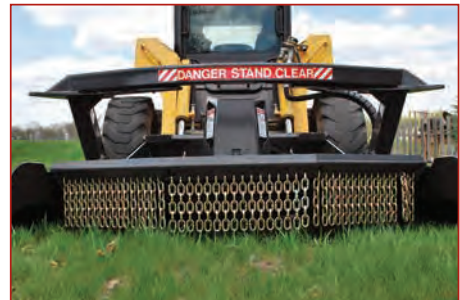
Heavy duty push bar pushes trees away from the operator while enhancing the cutting action by weakening the tree trunk as it bends.
