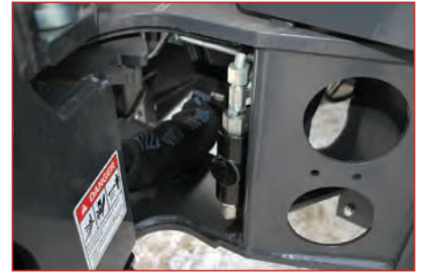
A standard flow control valve limits the oil flow to allow for optimal operating speed (optional on 485 model).
