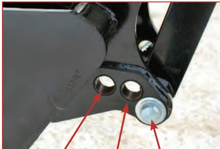
"Bell Hole" position allows bucket to open further and extend bucket reach
